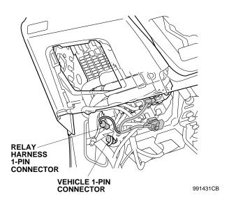
38. Remove lower hood opener bolt, and secure the relay bracket to the vehicle panel with the hood opener bolt.
