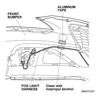
27. Secure the fog light harness to the front bumper with one aluminum tape.
