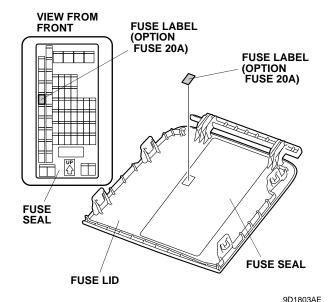
48. Using an isopropyl alcohol on a shop towel, thoroughly clean the fuse lid where the blank fuse label will attach. Attach the fuse label to the fuse seal of on the fuse lid as shown.
