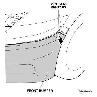
Release four retaining tabs on each side of the bumper.
