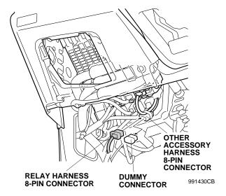
37. Plug the relay harness 1-pin connector into the vehicle 1-pin connector.
