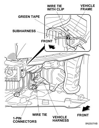
33. Secure the 1-pin connectors to the vehicle harness with one wire tie.
