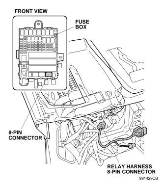
NOTE: If the 8-pin connector is already used by other accessory, locate the 8-pin connector taped to that other accessory harness. Remove the tape and dummy connector from that other accessory harness. Plug the fog light harness 8-pin connector into that other accessory harness.
