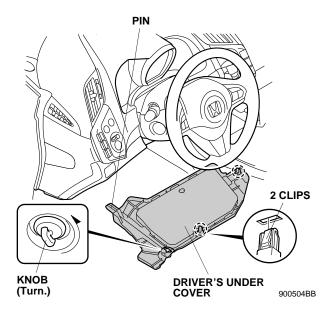
5. Insert a flat-tip screwdriver into the guide on the under side of the steering column lower cover and release the retaining tab.
