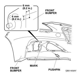
13. While wearing eye protection, drill the pierced mark in the front bumper with a 3 mm drill bit.
